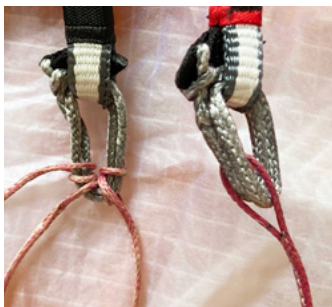
Left: loops on softlinks Right: loops released
