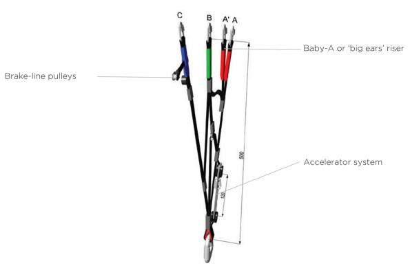
The riser set does not have trimmers, or any other adjustable or removable device.
